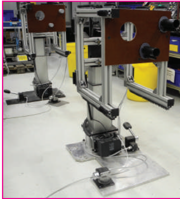
Electronic modules have push-button lift, and rotary modules are operated by two foot switches.
