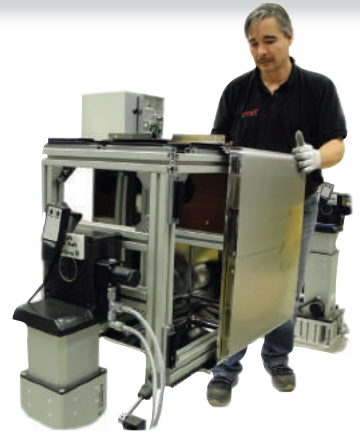
To protect the work surfaces, a clamping device with brushes on bearing surfaces holds inner containers.
