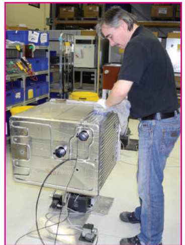
An employee covers five sides with heater foils, so the container has to be rotated several times.
