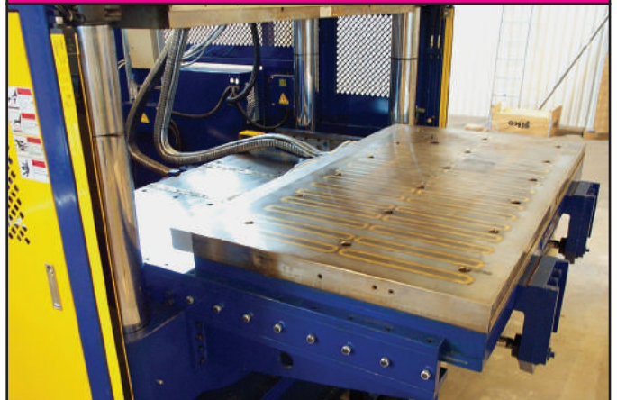
Figure 3 - 500 ton vertical press with lower roll out magnetic platen
