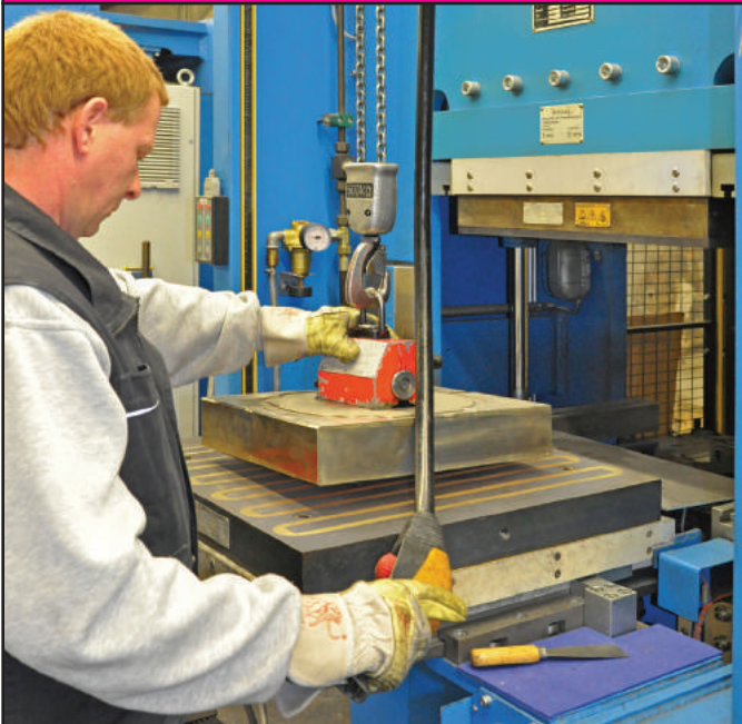
Figure 4 - mold lowered onto platen, magnetically clamped in seconds without tools or mechanical clamps
