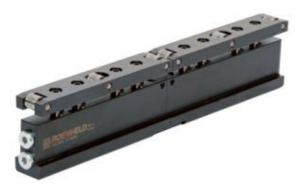
Double T clamps are for clamping on the bed or slide if mating T-slots are cut in the tool as well as the bed or slide. If the double T clamps are equipped with rollers, the die can be rolled into the press on these dual purpose roller/clamps.
