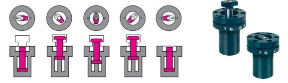
For clamping on the press bed or slide, this clamp provides unobstructed die movement since the clamping head pulls below the surface during die change. Proximity switches monitor the clamp, unclamp and changeover positions.
