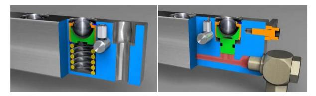
Roller Lifters: The use of dual direction rollblocks allow movement either front to back or left to right. Roller lifters have twice the lifting capacity of a ball lifter with about one half of the rolling resistance (1 to 3%). Since the load on the lifter is distributed across the roller there is not an issue with brinelling on the bottom of the subplate.
