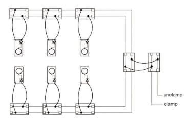
Pilot operated check valves providing a dual diagonal hydraulic safety circuit also ensure safe clamping for either the bed or the slide.
