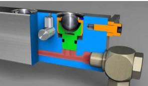
Ball Lifters: Ball type lifters allow movement in any direction. They have rolling resistance of 2 to 4% of the die weight depending on the surface condition such as hardness, smoothness, holes, etc. If the die weights are over 1,000 to 1,500 pounds, it is recommended to harden the bottom of the die or install hardened wear strips. This reduces the tracking (or brinelling) possible with the single point ball contact.
