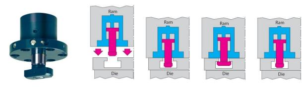
The swing clamp is for clamping the upper tool on the press slide. It can be recessed into pockets machined in the press slide or when provided with an extended shaft, the clamp can be mounted above the slide ledge. Proximity switches monitor the clamp and unclamp positions.
