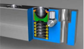
Hydraulic Lifters: Hydraulic lifters can support light or heavy dies during the die movement. Once in position, the die is simply lowered onto the bolster. To protect the operator and the equipment, a circuit relief valve should always be a part of the hydraulic circuit in case the rollblocks are accidentally overloaded.
