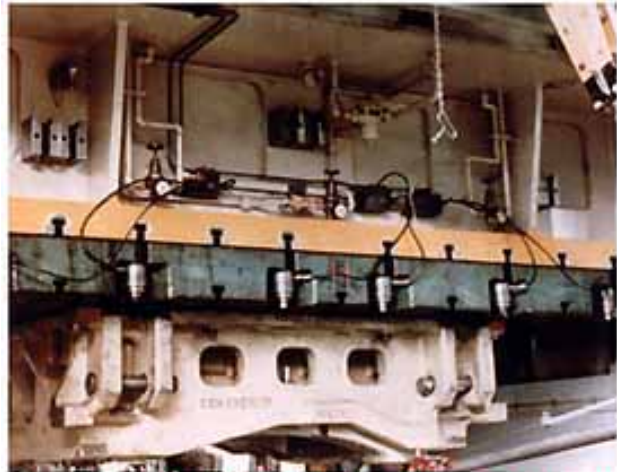
Hollow-piston clamps used in the press's existing T-slots can be positioned manually and installed in holders during die change.
