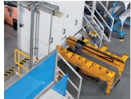
Die changing console with drive and side loading of the press.
