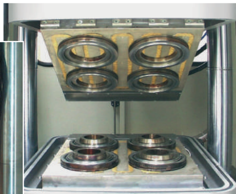
M-TECS 240 on a vertical press – various molds on a machine bed without loss of space due to clamping claws
