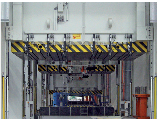
Clamping elements for a large transfer press, manufacturer Schuler
